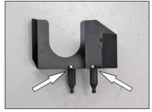
9. Attach the two stand-offs to the bottom of the  $K\&N^{\circ}$  heat shield as shown and secure with the hardware provided.
