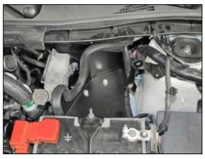
12. Install the heat shield into position on the air box mounting grommets as shown. **NOTE: Do not secure the bracket at this time.**
