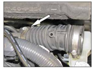
8. Loosen the hose clamp securing the intake hose to the turbo inlet and then remove the intake hose from the vehicle.
