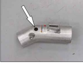
14. Install the provided grommet into the K&N $^{\otimes}$  intake tube as shown.
