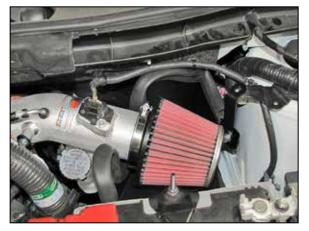
22. Route the mass air sensor wiring harness around the rear of the heat shield and then connect the mass air sensor electrical connection.
