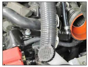
18. Install the tube mounting bracket (083164) onto the location from step #17 and secure with the provided hardware.
