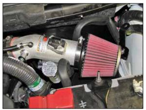
21. Install the K&N  $^{\mbox{\tiny ®}}$  air filter onto the intake tube and secure with the provided hose clamp.
