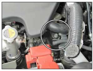
17. Remove the 6mm cover bolt shown.
