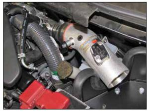
19. Install the K&N<sup>®</sup> intake tube into the coupling hose at the turbo inlet and align with the mounting bracket. Then secure the intake tube with the provided hardware and hose clamp.
