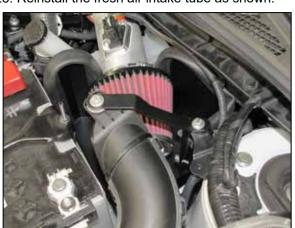
24. Secure the fresh air intake tube with the provided bracket (064315) and hardware on top of the heat shield mounting bracket.
