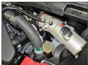
20. Insert the turbo waste gate fitting into the grommet installed into the K&N^ $\mbox{\ensuremath{^\circ}}$  intake tube. Use
