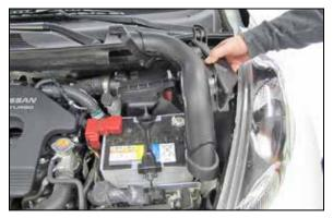
4. Pull up and release the fresh air intake tube and then remove the fresh air intake tube from the vehicle.
